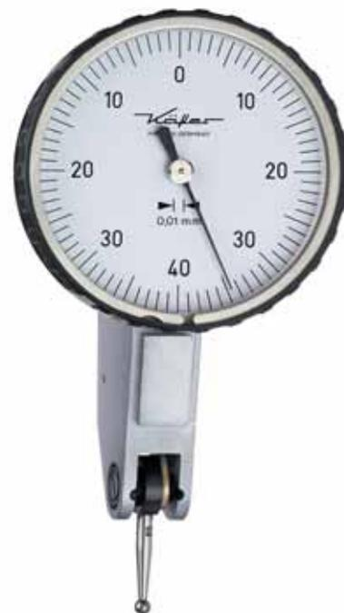
Dial Test Indicators are also available with extended measuring ranges of 1 mm or 2 mm. Please request our offer for the models K 30/1, K 30/2, K 40/1 and K 40/2.
