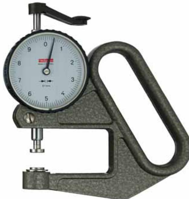
Model **K 50 with lifting device** has the same technical specification as model K 50 with pressure lever. At rest the contact points are closed. This style has the advantage that the contact pressure of 0.5 N is applied independently of the user. The **Spare Dial Gauge for K 50 with lifting device** will be supplied without lifting device unless requested on the order.
