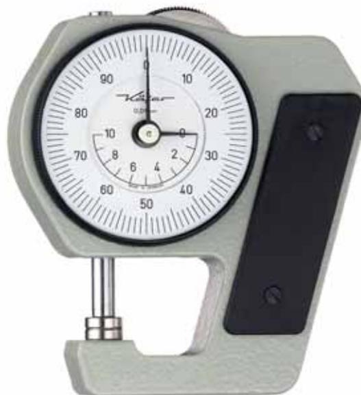
The contact points are in contact when the Pocket Dial Thickness Gauges J 12 and J 15 are not in use. The serrated lifting wheel opens them for the insertion of the component. The size can be easily read off the scale. The instruments can be zeroed by using the knurled adjusting bezel.
